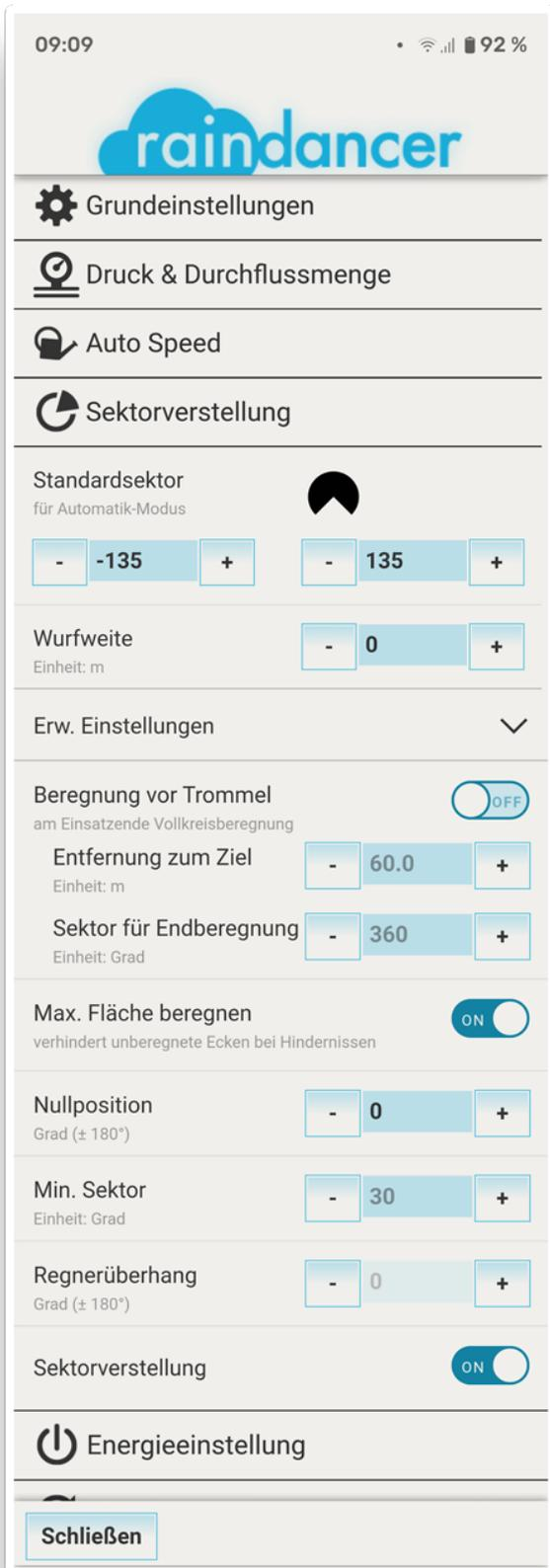
Click on the irrigator and go to the buttons **"More"** -> **"Settings"** -> **"Sector Adjustment"**, here you must "activate" (ON) the Sector Adjustment.
