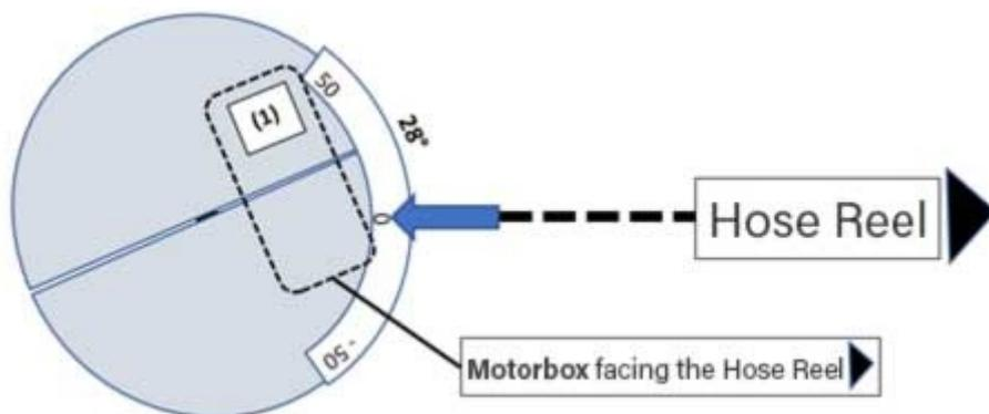
**Zero Position:** Please hold (or stick) the included sticker with the angle indication in a way that the zero mark points towards the hose reel. Now you can read off the zero offset at the groove between the cover plates (**here 28°**). Please take care to note if + or - (+28° or -28° for example).
