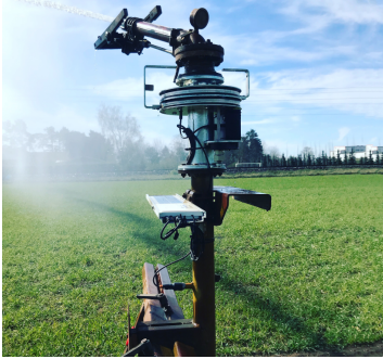
Mounting a Sector Control on a Irrigation Trolley.
